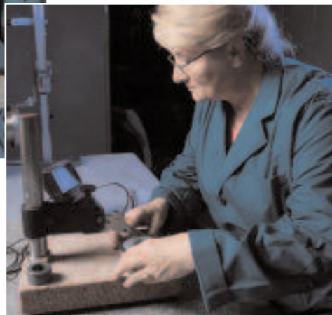
Technicians measuring the dimensions of pump components with precision calipers: Liquiflo pump components are precisely manufactured to tolerances as low as .0004 inches (10 microns).
