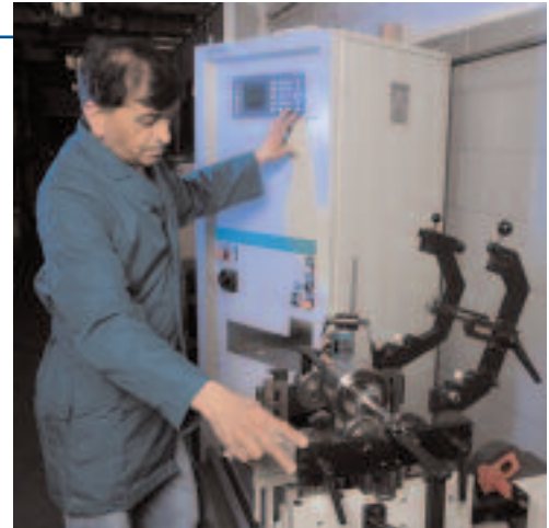
Technician balancing inner magnet for a mag-drive pump: Precision balancing of internal components significantly extends the service life of our products.
