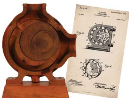
This wooden model was hand carved by Jens Nielsen. Its Gear-Within-A-Gear design was used to solve Nielsen’s water seepage problem and was the foundation on which the Viking Pump Company was founded.
