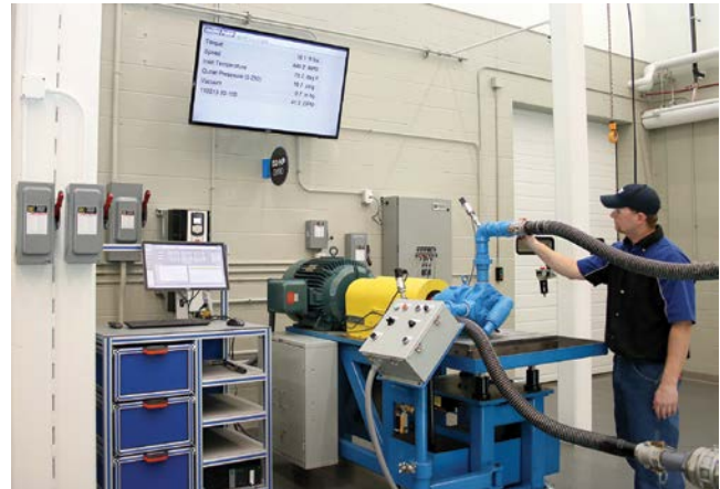
Certified performance testing on a sealless magnetically-coupled pump on one of 8 dynamometers in our newly expanded research lab, allows us to test a full range of pump capabilities on liquids at the customer’s viscosity.
